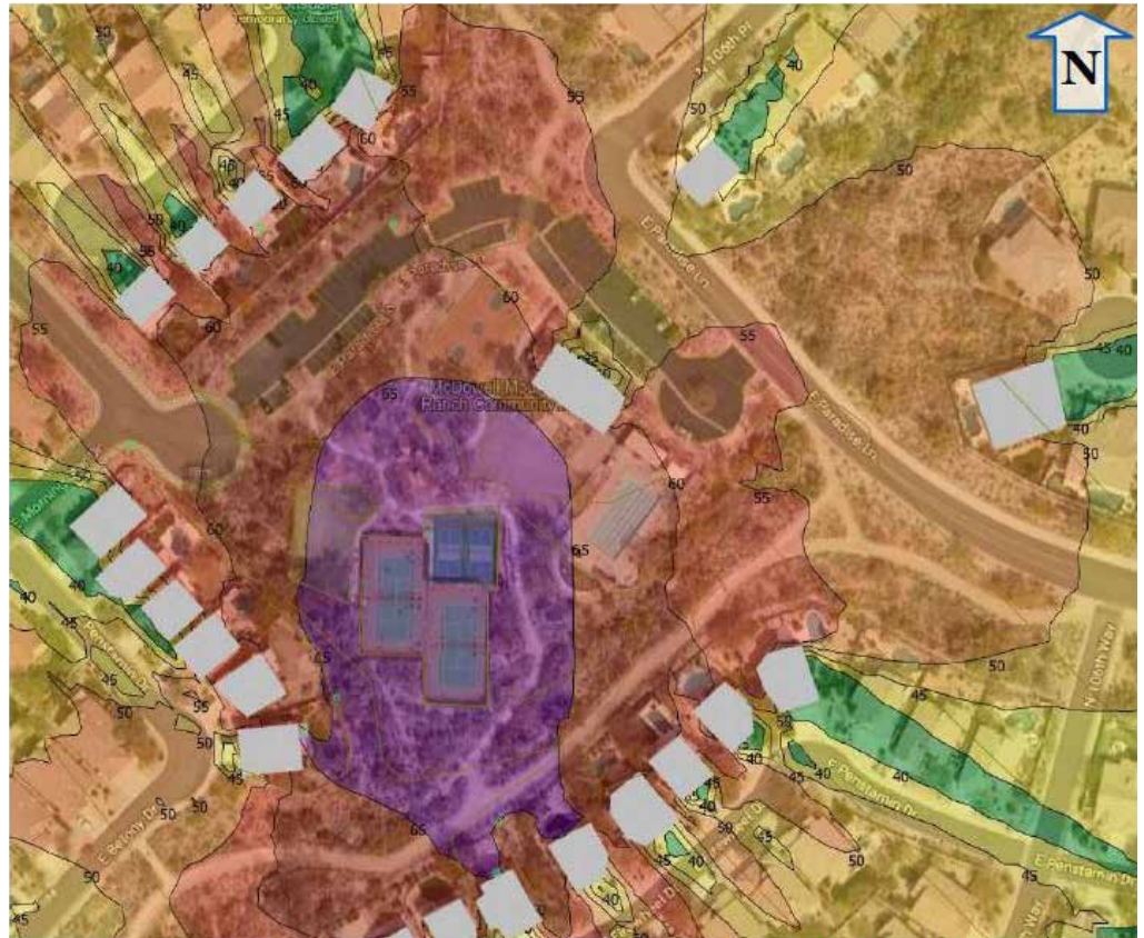
Figure 4.3. Adjusted Sound Pressure Level Contours for All Pickleball Courts
